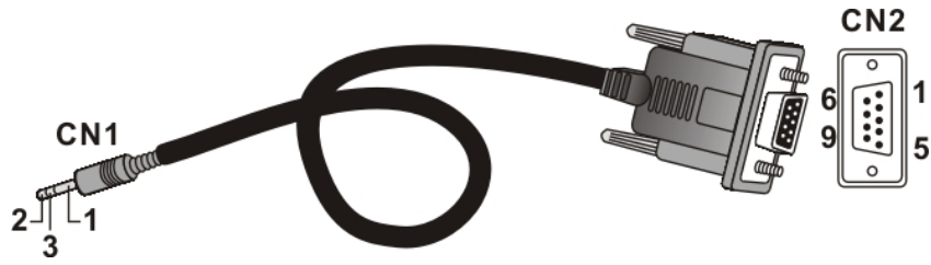
Figure C-4: Connector Pinouts - Adapter Cable for COM2
